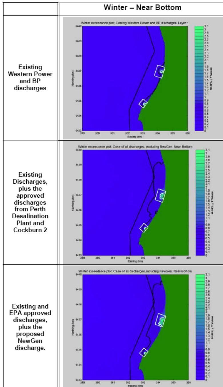
**Figure 8 Modelled spatial extent of temperature elevations in Winter near bottom layer (E2 boundary and contour is black lines, E3 boundary and contour is white lines) Note: Reference to Western Power means Verve Energy.**
