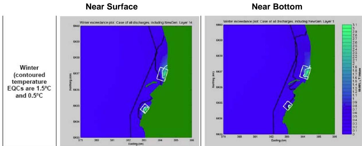
Figure 6 Modelled spatial extent of temperature elevations in Winter (E2 boundary and contour is black lines, E3 boundary and contour is white lines)
