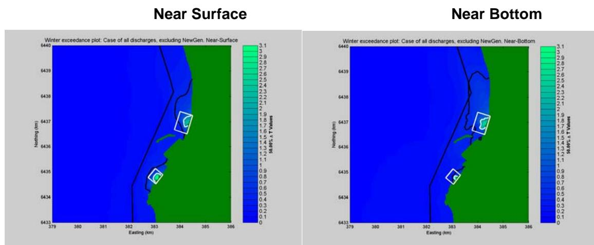
Figure 7 Modelled spatial extent of temperature elevations in Winter without NewGen outflow (E2 boundary and contour is black lines, E3 boundary and contour is white lines)
