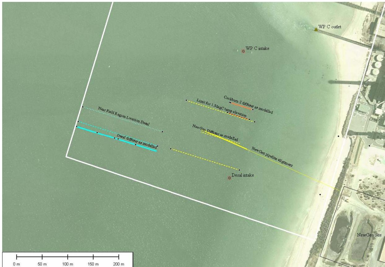
**Figure 2 Location of other modelled facilities adjacent to NewGen Power diffuser (yellow solid line) including other diffusers (solid lines) and intakes (black circles). White line is the boundary of the LEPA. Mixing zones indicated by dashed lines. Verve Energy stage A/B intake is some meters north of the WP C intake shown.)**
