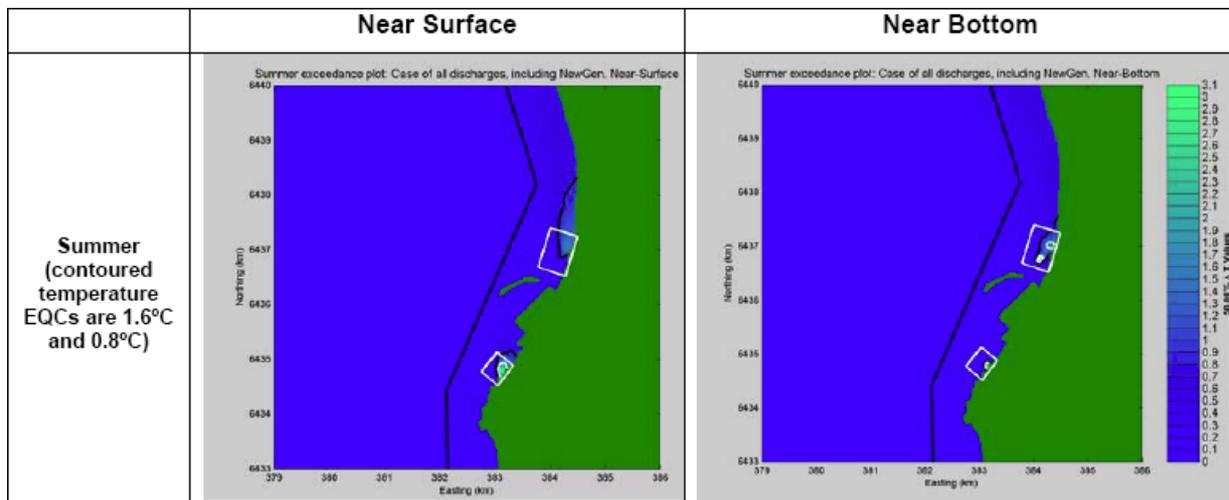
Figure 4 Modelled spatial extent of temperature elevations in Summer (E2 boundary and contour is black lines, E3 boundary and contour is white lines)
