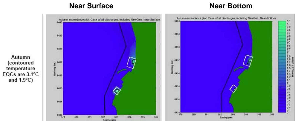
Figure 5 Modelled spatial extent of temperature elevations in Autumn (E2 boundary and contour is black lines, E3 boundary and contour is white lines)
