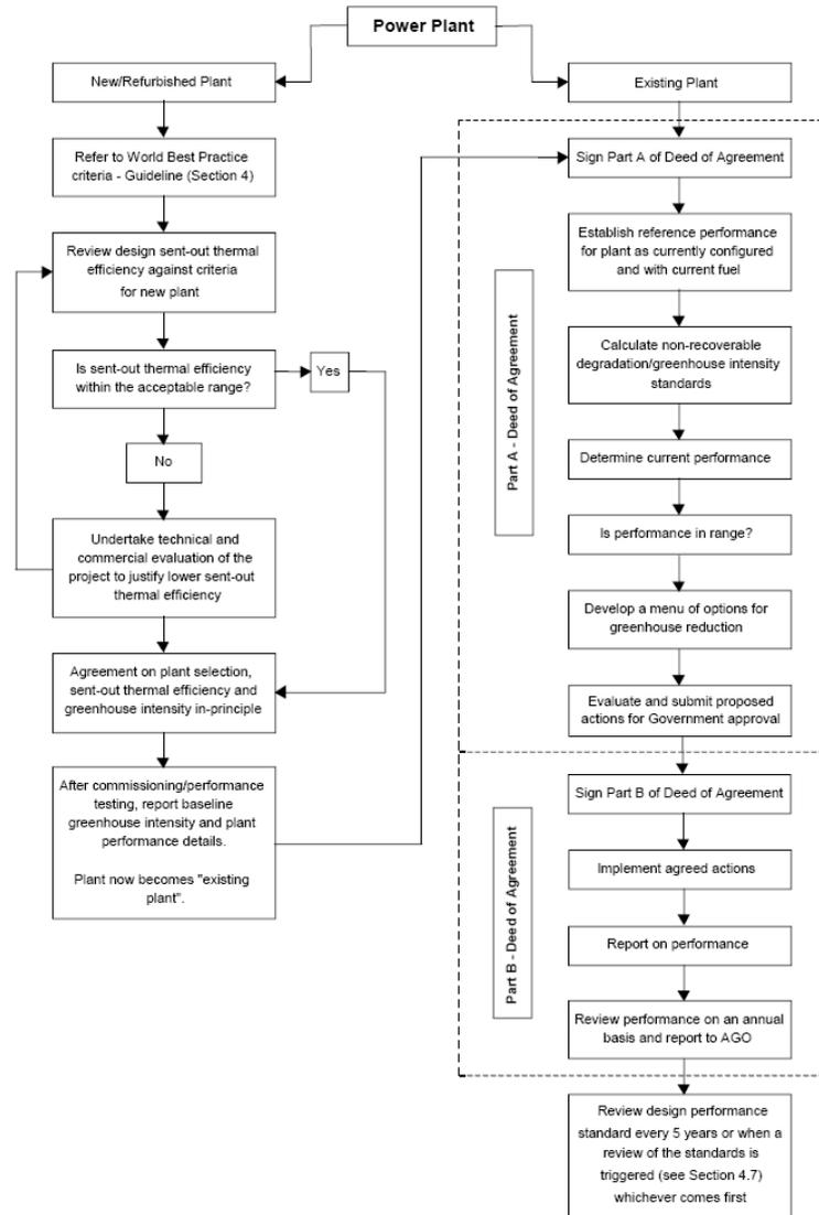
Figure 1 – Generator Efficiency Standards – Process flow chart
